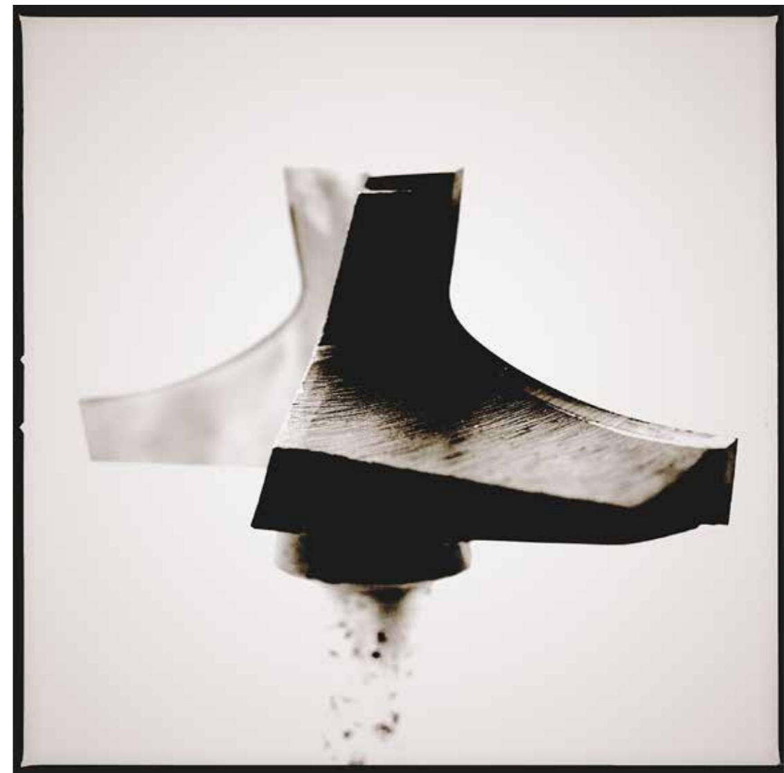
The blade of the NC router. Which is indispensable in making furniture of HIRASHIMA.
